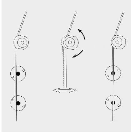
Refer to the screw in the center of the natural disk, which indicates the ideal position. You may choose a different position if this seems necessary. When the position is correct, tighten the screw firmly, maintaining the string nut in place.
