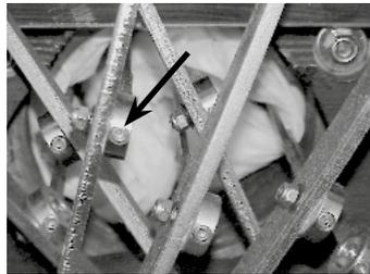
6. If the Rod-tuner gives off the high-pitched sound in natural, the cable must be shortened. To gain access to the area under the base, lay the harp in its side on a soft support, like a sofa or a padded bench, insuring that the Rod-tuner is not touching anything, or bearing any of the weight of the instrument.
