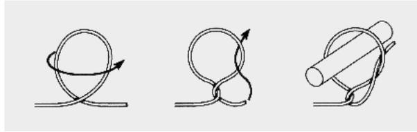
3. Here is a description of how to knot the end of the string. Pass the wooden dowel into the loop of an overhand knot in the end of the string, and then tighten strongly. For the higher strings, you can make an overhand knot with an extra initial loop, which will make the knot hold tighter. You can also make an additional loop around the dowel for the highest strings, which prevents unravelling until the string is under tension.
