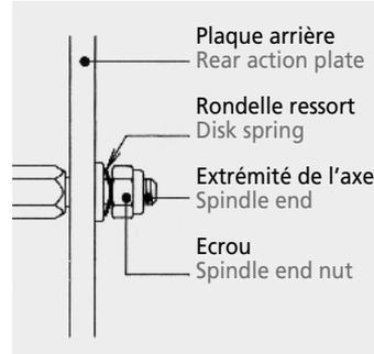
To check: To determine for certain if this is an action plate buzz, try to press on the disk at the same time as the string is plucked. The force from pushing on the disk should prevent the disk from buzzing. If this is the case, the buzz ceases.
